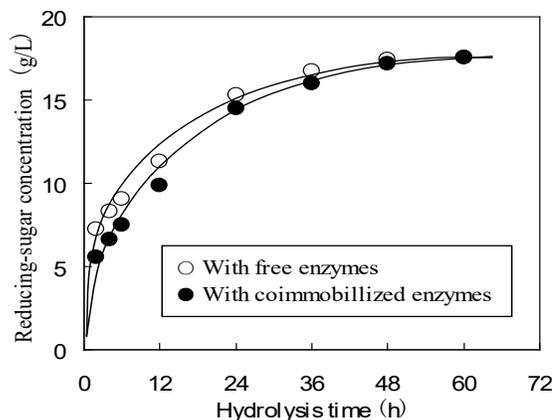
**Figure 3.** Changes of reducing-sugar concentration during the hydrolysis of pretreated rice straw with free and coimmobilized enzymes.
